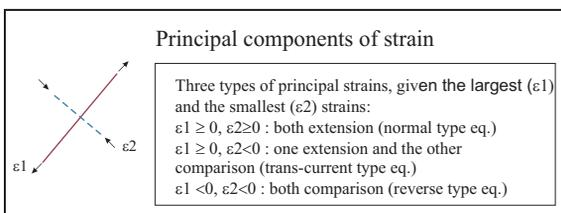
Figure 10. The strain component and constituent mechanisms (Kato, 2011).
