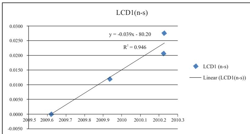
Figure 4. Displacement rate of N-S (north-south) component of LCD1.
